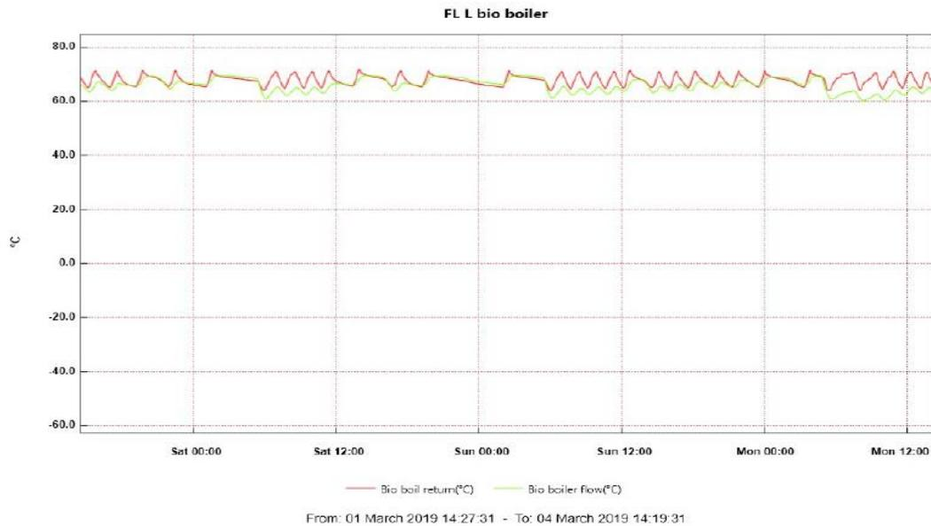
Note the evidence of ‘cycling’ of the boiler at frequent intervals.
