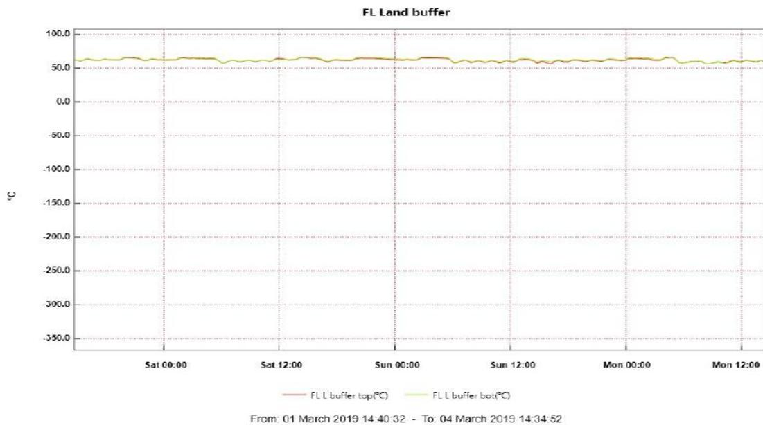
Note above the lack of any real temperature differentiation between flow and return of the buffer tank. The tank exists as a virtual pass-through of hot water with only a short delay in the tank.
