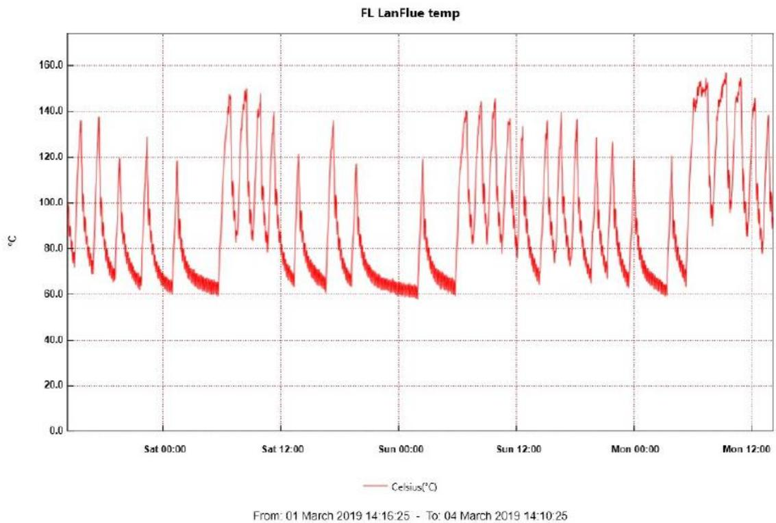
Note the frequent fluctuations in flue temperatures as the boiler cycles frequently and drops down to low kindling-slumber mode. This is mirrored in the O<sub>2</sub> levels shown below.
