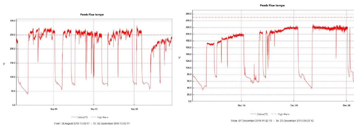
As can be seen in Figure 4 there is a slow and steady upwards drift in the boiler exhaust flue temperatures over the month between heat exchanger cleaning. This indicates a slow deterioration in the efficiency of heat exchange between the boiler tubes and water jacket surrounding it. In summary an increasing amount of energy from the wood fuel is ending up as wasted heat via the exhaust flue.
