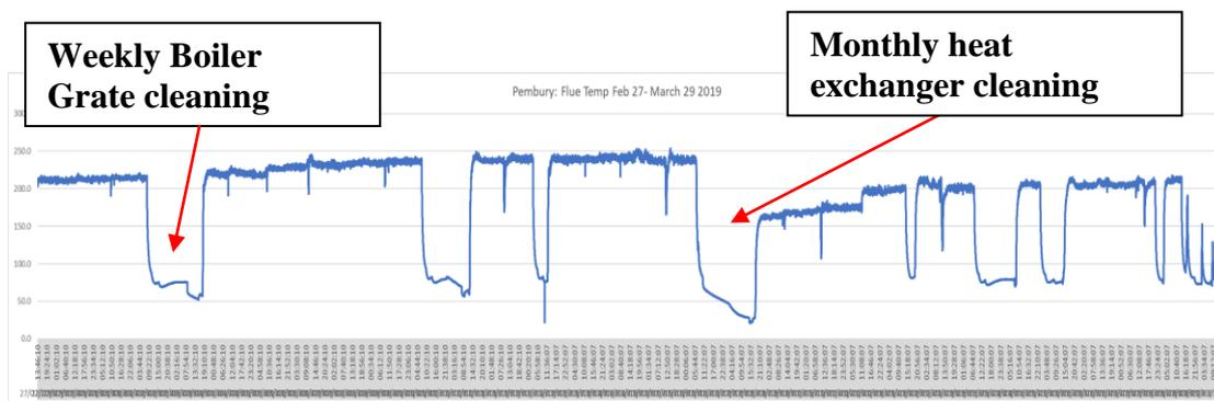
**Figure 4: Increased cleaning reduces flue temperatures from 250°C to 200°C**
